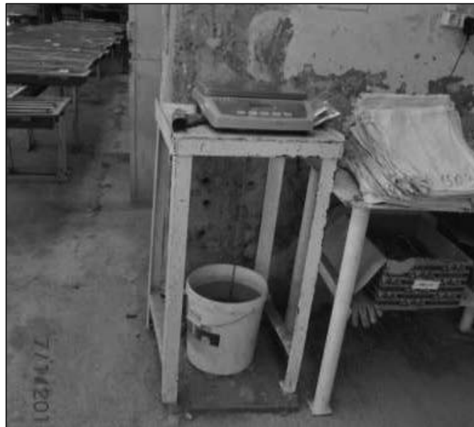
Figure 12: Density measurement weigh balance. CSA Global visit September 2018.
