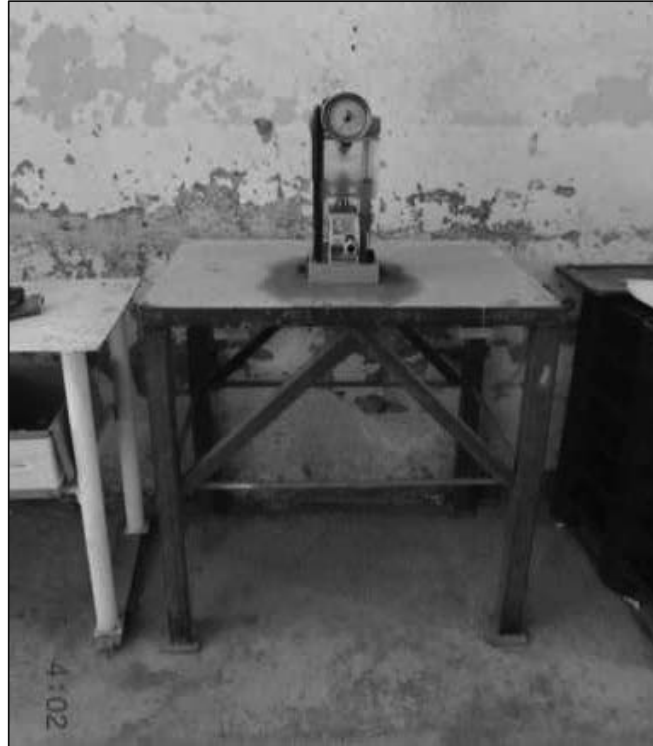
Figure 13: Point load balance. CSA Global visit September 2018.
