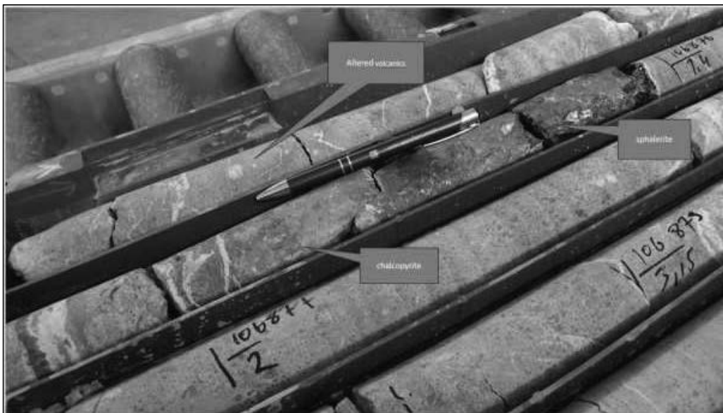
Figure 6: Mineralisation from definition drilling in September 2018 with Sphalerite and chalcopyrite).
