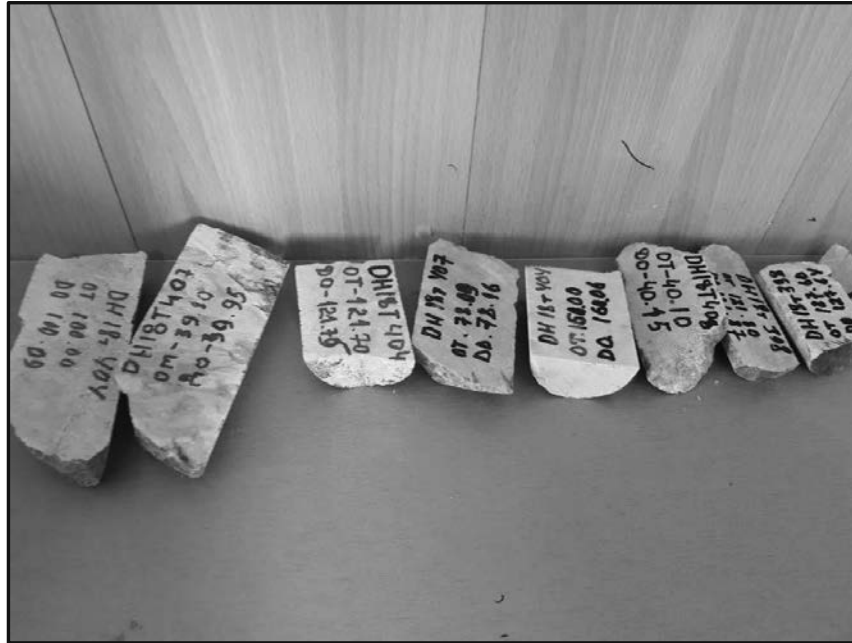
Figure 3.20 Samples for Density Determination
